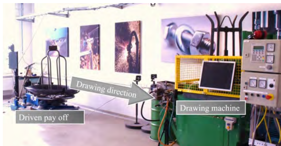
Figure 1. Research wire drawing line at Örebro University.
