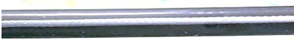
Figure 6. Shallow artificial scratch after being reduced in the drawing die.
